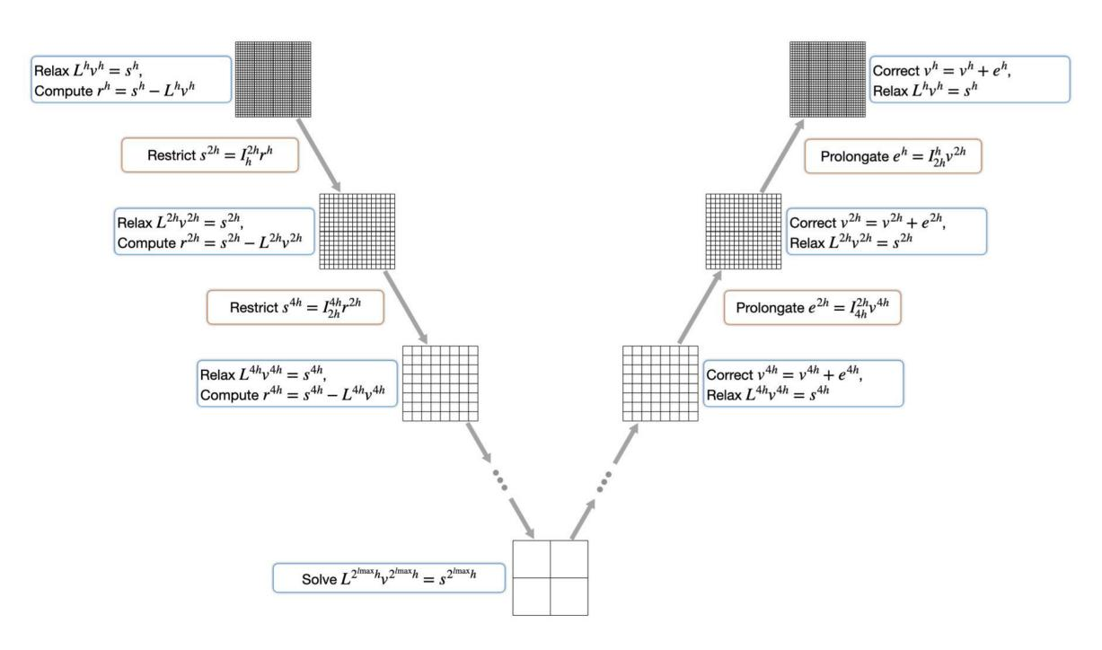
Multigrid is one of the optimal technique for solving elliptic partial differential equation by adopting hierarchical grid system to accelerate the convergence of relaxation method as shown in Figure 1.
